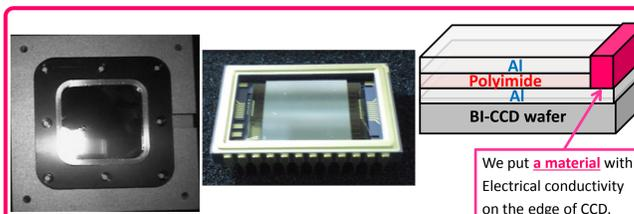
Fig 2. (Left) : Picture of Suzaku OBF. The size of this OBF is  $\sim 3\text{cm} \times 3\text{cm}$ . The silver area is the OBF inside the black frame.
