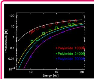
Fig6. The red circle and green square shows the EUV transmission of Polyimide, with  $2400\text{\AA}$  and  $3000\text{\AA}$  thickness, respectively.
