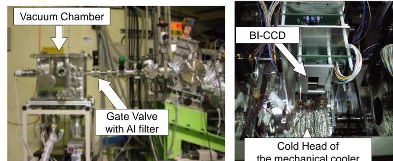
Fig 4. (Left) : Set up at BL-20A in KEK-PF. EUV light is radiating from the right hand side in this picture. (Right) : CCD in the vacuum chamber. The vacuum level and CCD temperature was  $10^{-7}$  mbar and  $-55$  deg, respectively.
