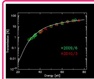
Fig7. The white line is the modeled transmission curve assumed the thickness of polyimide to be  $\sim 1100\text{\AA}$  (design value). We found there was not difference of the EUV transmission during 9 month comparing the first and second experiment at KEK-PF (red circle and green square).
