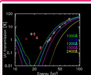
Fig5. EUV transmission of the polyimide of OBL. Five lines show the calculated transmission. For example, we assumed the thickness of polyimide is  $1100\text{\AA}$  which is derived from the design value. There is the residual below 23eV, where the data are affected by the contamination of the higher order light at the beam line.
