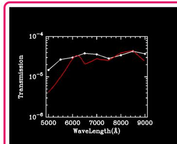
Fig8. Optical transmission of OBL. The white circles is result of our experiment, and the red line is assumed the thickness of Al is  $\sim 50\text{\AA}$  and  $800\text{\AA}$  which is thinner value than the design value (see table2). The expected optical transmission was less than  $10^{-5}$  in the visible range. This discrepancy might be caused by the oxidation of Al which was reported by the previous work [1,2].
