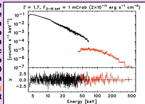
Fig.2 HXJ (black) and SGD (red) simulation results for a 100 ks observation of a source with with 1/1000 of the Crab brightness and power law index of 1.7
