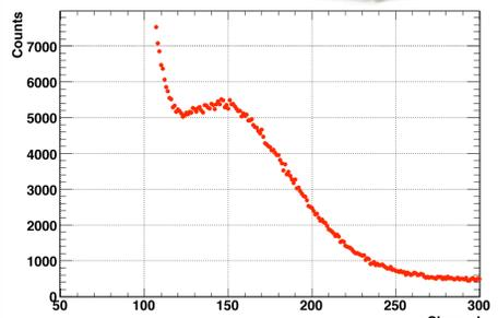
Fig. 6 <sup>241</sup>Am spectrum from APD with a BGO similar in shape as the one in the SGD shield.
