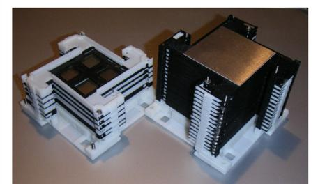
Fig. 5 Pictures of mechanical models for SGD Compton camera. The model on the right survived a vibration test.
