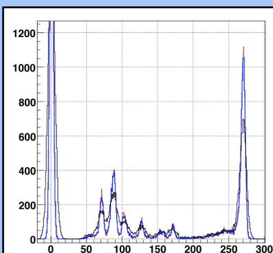
Fig.4 <sup>241</sup>Am spectrum from a CdTe sensor readout by an ASIC with on-chip digitization. Comparison of spectra without CMN subtraction (black), with on-chip CMN subtraction (blue) and with off-line CMN subtraction (red).
