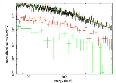
Fig. 3 SGD simulation results for a 100 ks observation of bremsstrahlung emissions from Cas-A with three magnetic field hypotheses, 0.1 mG (black), 0.3 mG (red) and 1.0 mG (green).
