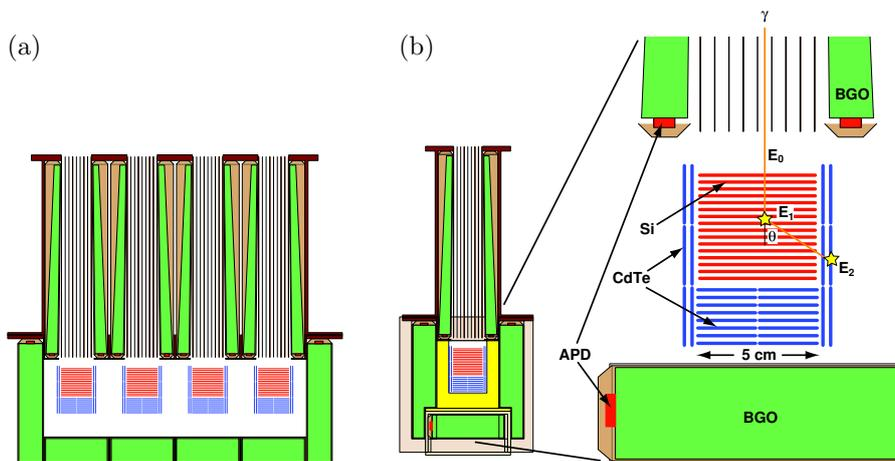
Fig. 1.1. Conceptual drawing of (a) an SGD instrument and (b) an SGD Compton camera unit.
