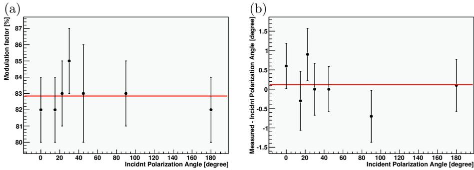
Fig. 1.5. (a) Modulation factor as a function of the polarization angle. (b) The difference between the polarization angle derived from the experimental data and that of the incident photons as a function of the incident polarization angle.
