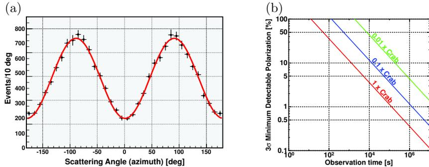
Fig. 1.3. (a) Efficiency-corrected azimuth angle distribution of Compton scattering from a source with a brightness of Crab and 100% linear polarization in a 10 ks observation. (b)  $3\sigma$  MDP as a function of observation time for sources with 1, 0.1 and 0.01 of the Crab brightness.
