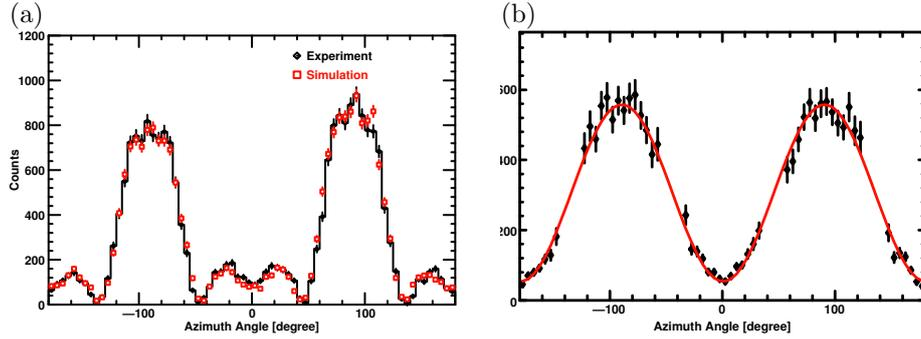
Fig. 1.4. (a) Comparison of experimental (black solid diamond) and simulation (red open square) results of the azimuth angle distribution without any instrument response corrections. (b) Experimental azimuth angle distribution with instrument response corrections obtained from the MC simulation with a model fit.
