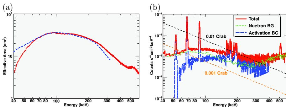
Fig. 1.2. (a) Effective area as a function of incident energy. (b) Background flux as a function of reconstructed energy.
